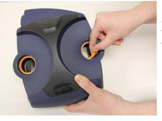
**11.1** The gasket has a groove all round and is fitted on a flange below the threads in the filter mounting.
