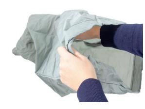
**6.2** Turn the flow meter bag inside out so that the transparent measuring tube is on the outside.
