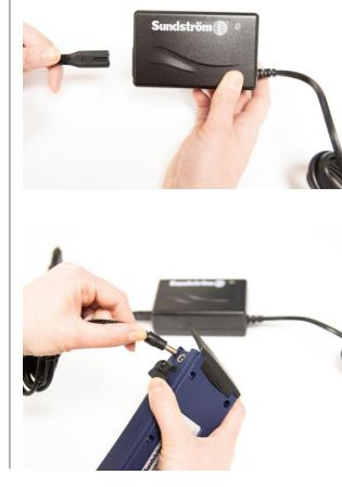
**1.3** Connect the power supply lead to the battery charger. Connect the battery to the battery charger. Connect the power supply lead of the charger to the wall socket.
