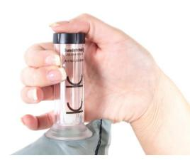
**7.1** Cause a flow stoppage by still holding tightly the joint between the hose and the flow meter bag and then blocking off the flow meter outlet.
