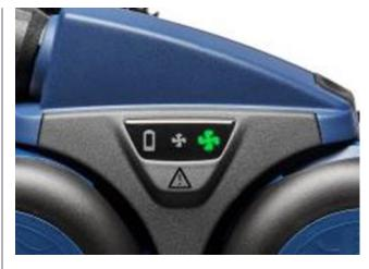
**5.3** If the button is pressed again, the flow will increase to 240 l/min, and this is indicated by the large fan symbol lighting up. If the control button is pressed again, the fan flow rate will revert to 175 l/min and the small fan symbol will again light up.
