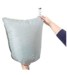
**6.3** Place the head top in the flow meter bag and start the fan unit.
