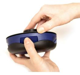
**9.1** Change particle filter by bending the pre-filter holder from the filter adapter.
