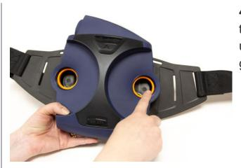
**4.3** Check that the gaskets in the filter mounting of the fan unit are in place and are in good condition.
