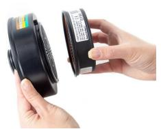
**9.4** To change the gas filter: Unscrew the filter/combined filter. To change the gas filter, prise the particle filter off the gas filter. Bear in mind that both filters/combined filters must be changed at the same time and must be of the same type and class.
