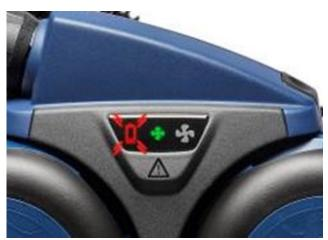
**5.5** When about 5% of the battery capacity is left, the fan will begin to initiate an alarm and the battery symbol will flash. The battery capacity is sufficient to allow the work to be concluded without undue haste. The work should then be interrupted and the wearer of the equipment should leave the site.
