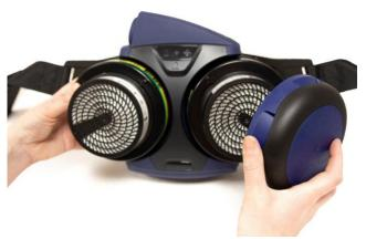
**4.5** Screw the filter combination into the filter mounting so far that the filter will be in contact with the gasket. Then turn it about 1/8 turn further in order to ensure a good seal. Press the filter holder onto the particle filter. The filters used must be of the same type, i.e. two SR 510 P3 or two SR 518 A2/SR 510 P3, etc.
